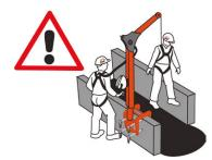
Working Load Limit: 1 person weighing a maximum of 136kg including all clothing, tools and equipment connected to the HRA / Winch. The operator of the winch needs to be connected to the secondary anchor point on the mast using a type 3 SRL.
