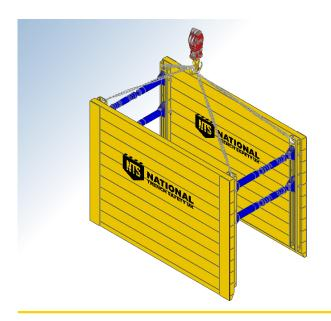
After standing upright check all pins and safety clips are in place. Lift the box using the four leg chain sling attached to the lifting points at the top of each panel.
