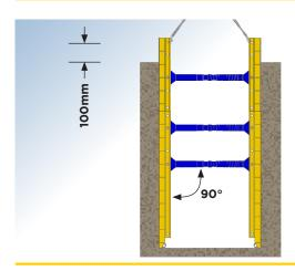
Continue the dig and push operation until the required excavation level is reached. Ensure all the struts are horizontal and at right angles to the panels before entering the excavation.
