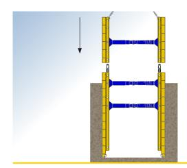
Align the top box and lower into position over the Base Box. Ensure connectors locate in top panel end posts.
