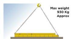
Lie first base panel flat on ground with spindle connector points upwards.
