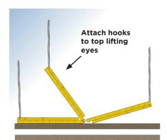
Turn the other base panel over using 2 legs of the four leg sling.
