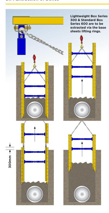
Due to the consolidation of the ground against the modules, it is usually more difficult to extract Lightweight Box Series **300 or Standard Box Series 600 than to insert** them. Methods for extracting are as follows, remembering that all lifting must be done at the points provided.
