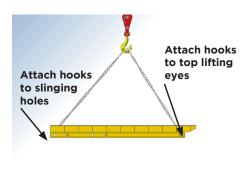
Re-sling this panel with the wings downwards (Use all 4 legs of the lifting chain)
