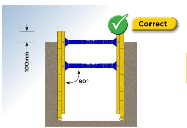
When the required excavation level is reached and the box sunk to full depth, ensure that the struts are horizontal and at right angles to the panels before entering the trench.
