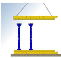
Complete assembly of the base box on it's side by pinning the struts to the upper panel. Remove the 4 leg sling.
