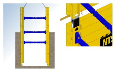
Attach the top box to the base box using box connectors and Ø 20\*150 mm pins & 'R' clips.
