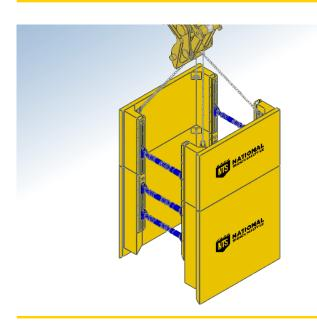
After standing upright check all pins and 1 safety clips are in place. Lift the box using the four leg chain sling attached to the lifting points at the top of each panel.
