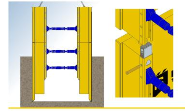
Attach the top box to the base box using box connectors and Ø 20\*150 mm pins & 'R' clips.
