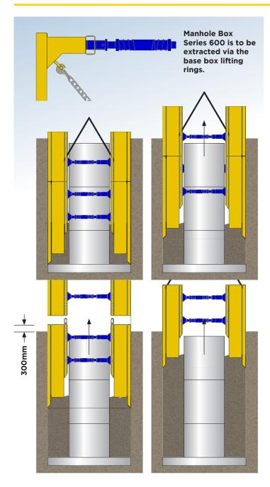
Due to the consolidation of the ground against the modules, it is usually more difficult to extract Manhole Box 600 boxes than to insert them. Methods for extracting are as follows, remembering that all lifting must be done at the points provided.
