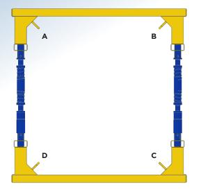
Dig the manhole approx. 600-1000mm 2 deep to the correct width, and using the four leg sling place the box in the excavation.
