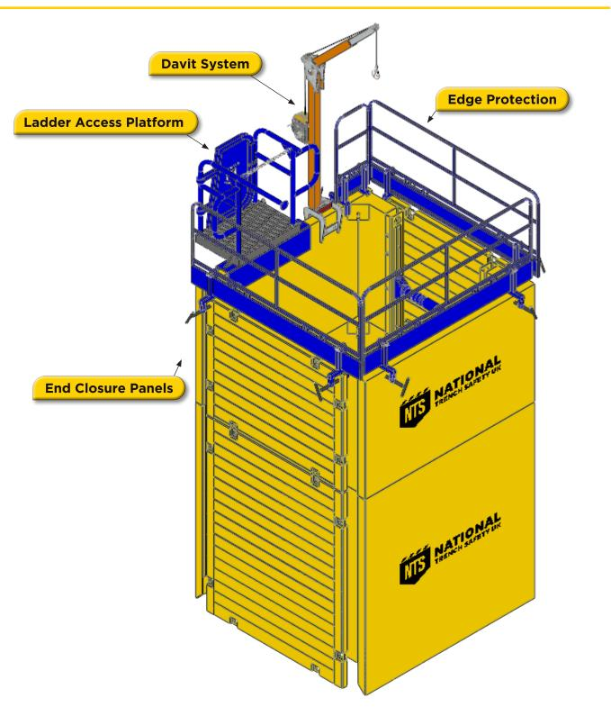
NOTE: DON'T FORGET YOU WILL NEED A LADDER, LADDER ACCESS PLATFORM, DAVIT SYSTEM AND EDGE PROTECTION TO COMPLETE YOUR INSTALLATION.
